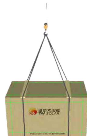
Figure 6 Schematic diagram of Module lifting
