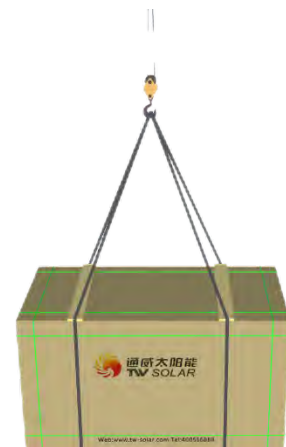
Figure 6 Schematic diagram of Module lifting
