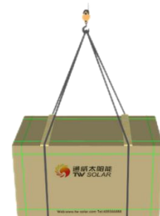
Figure 6 Schematic diagram of Module lifting
